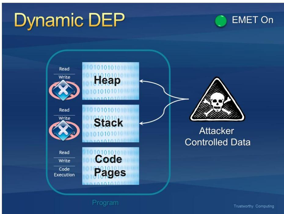
Figure 4: DEP blocking shellcode from running
